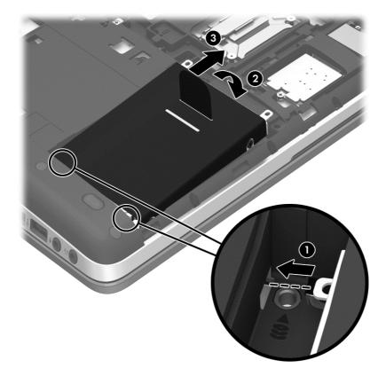
3. Tighten the 4 hard drive screws to secure the hard drive.
