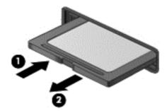
**NOTE:** If the card is not ejected, pull the card out of the slot.
