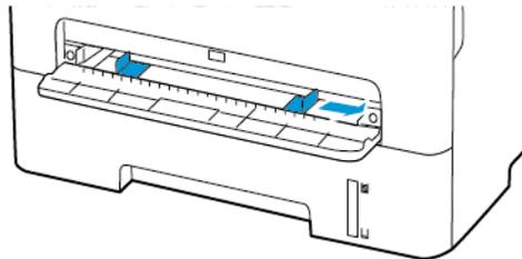
3. Load a sheet of paper with the printable side face-up.
